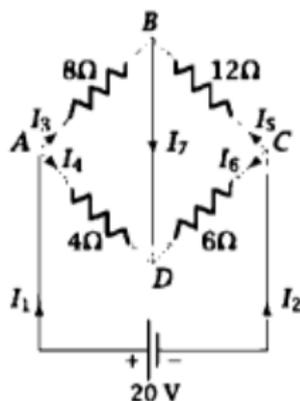
If the ratio of the resistances to the left of the “bridge” BD is the same as the corresponding ratio on the right, there should be no current through the bridge. Thus, testing that  $I_7 = 0$  provides a way to be sure that the ratios are the same. Let us see if this is the case.
