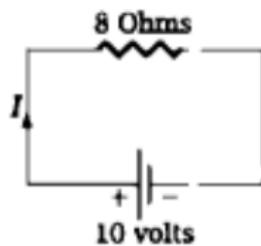
In a simple circuit such as the one shown above, Ohm's Law gives us two pieces of information. It says that the size of the current flowing around the circuit is  $I = \frac{E}{R} = \frac{10}{8} = 1.25$  amps. It also gives us the size of the voltage drop at the resistor:  $V = IR = 1.25(8) = 10$  volts.
