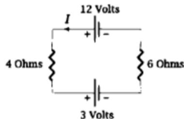
A basic principle due to Gustav Kirchhoff (1824-1887) says that the sum of the voltage drops at the resistors on a circuit must equal the total voltage provided by the batteries. For the circuit on the left of the above, the voltage drops are  $4I$  at one resistor and  $6I$  at the other for a total of  $10I$ . The total voltage provided by the batteries is  $3 + 12 = 15$ . Kirchoff's Law says  $10I = 15$ , So the current around the circuit is  $I = \frac{15}{10} = 1.5$  amps.
