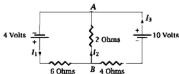
At  $A$ , there are two entering currents of  $I_2$  and  $I_3$  amps and a single departing current of  $I_1$  amps. At  $B$ , the entering current of  $I_1$  amps splits into currents of  $I_2$  and  $I_3$  amps.
